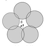
Figure 6. A coverage patch bounded by arcs of sensing circles
