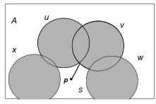
Figure 7. A coverage patch bounded by arcs of sensing circles and boundary of a coverage region
