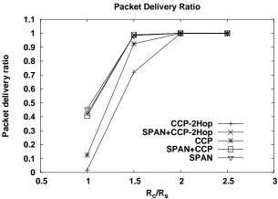
Figure 15. Packet Delivery Ratio vs. Rc/Rs
