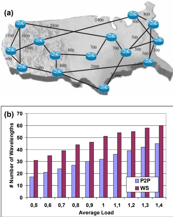
Figure 5: (a) 14-node NSFnet backbone network topology (the shown distances are in km) and (b) number of wavelengths per average load needed to support the communication of all source-destination pairs with shortest path routing in the case of wavelength switching (WS) and point-to-point packet switching (P2P), for 0.01 loss ratio.
