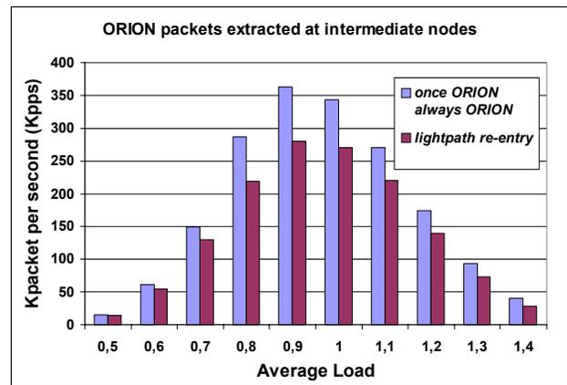
Figure 9: Number of packets uploaded at intermediate nodes.
