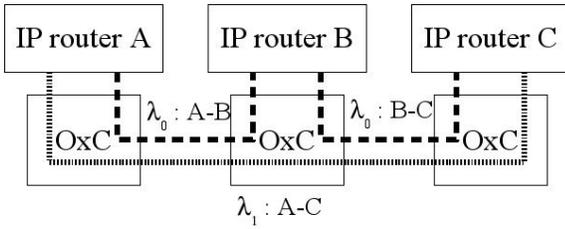
Figure 1: ORION switching paradigm: In the case that  $\lambda_0$  wavelength channel of A-to-B connection overloads, packets from A to B are sent in “overspill” mode over  $\lambda_1$  wavelength channel, although  $\lambda_1$  is a direct wavelength path from A to C.
