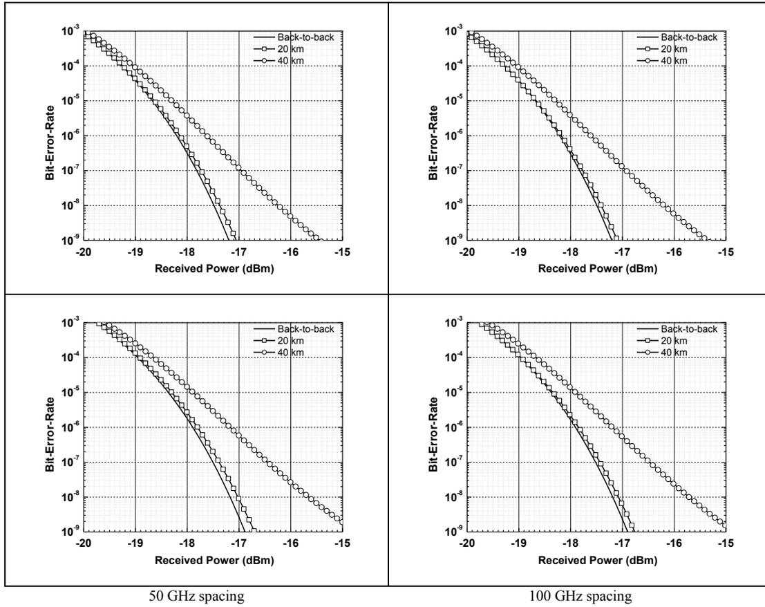
Figure 3. Physical layer performance evaluation for the WDM-based PON architecture. The number of wavelengths equals 64 (top row) and 128 (bottom row).
