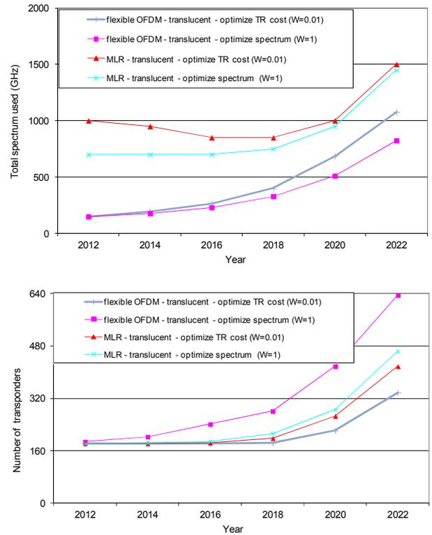
Figure 2: (a) Maximum spectrum used (GHz), and (b) transponders' cost, for the flexible and the MLR network, for optimizing the maximum spectrum used ( $W=1$ ) and the transponders' cost ( $W=0.01$ ) on the DT network.
