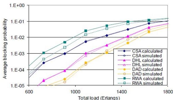
Figure 4: Blocking performance of the different SEC polices for the flexible optical network and a WDM network.
