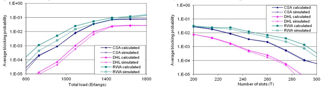
Fig. 6: Average blocking probability vs. (a) the total load, assuming  $T=250$  slots and (b) the number of slots  $T$ , assuming 1000 Erlang load.
