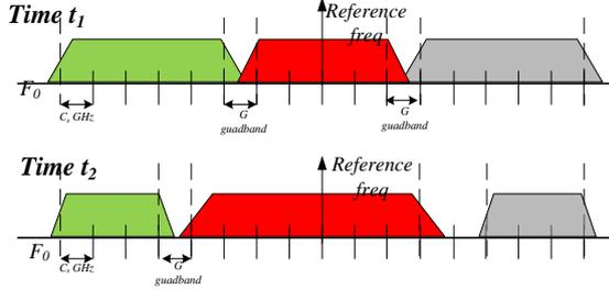
Fig. 1: Spectrum allocation of a link's bandwidth to variable rate connections. Two different time instants are displayed in (a) and (b). Spectrum guardabands of  $G$  slots separate the connections so that they are routed and received with acceptable BER.
