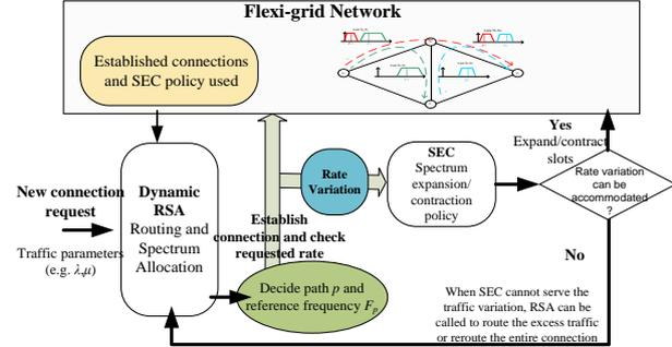
Fig. 2: Flow diagram for serving a connection request. Dynamic RSA is used to determine the path and reference frequency and SEC policy takes care of traffic variations.
