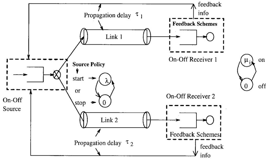
Fig. 2. Framework for multicast flow control.
