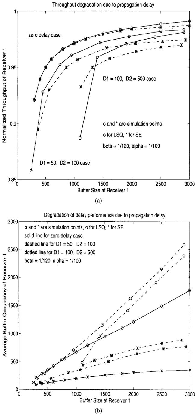
Fig. 8. Performance degradation due to propagation delay. (a) Throughput. (b) Average buffer occupancy.
