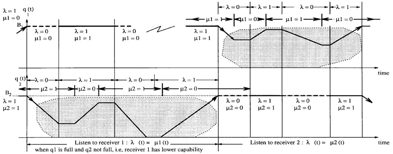
Fig. 4. Periodic evolution of the buffer occupancy for LSQ with zero delay.
