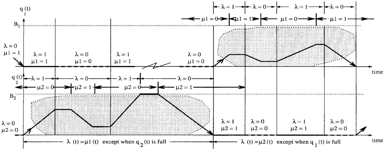
Fig. 5. Periodic evolution of the buffer occupancy for SE with zero delay.
