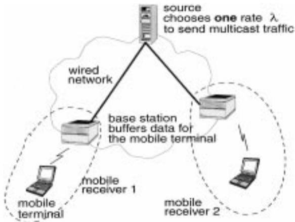
Fig. 1. Simple scenario for multicast.
