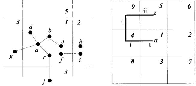
Fig. 5. Routing path i uses the interzone routing table, and path ii uses intrazone routing table.
