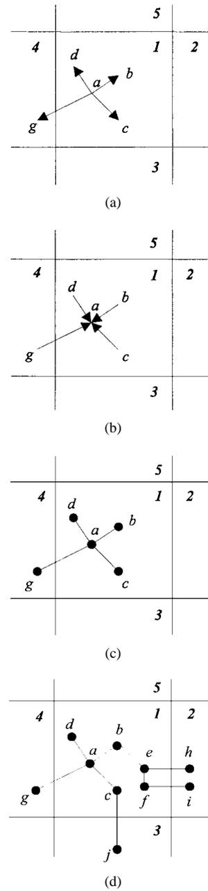
Fig. 3. Intrazone clustering procedure. (a) Node *a* broadcasts a link request to its neighbors. (b) Node *a* receives link responses from its neighbors. (c) Node *a* generates its own node LSP and broadcasts it throughout the zone. (d) All nodes perform the previous steps asynchronously.
