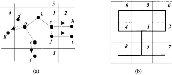
Fig. 4. Interzone clustering procedure. (a) Gateway nodes broadcast zone LSP's throughout the network. (b) Virtual links between adjacent zones are established.
