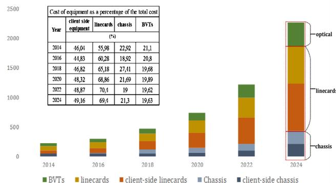
Fig. 6. CAPEX profile of a multilayer network
