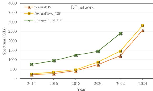
Fig. 5. Maximum spectrum used for the DT network.
