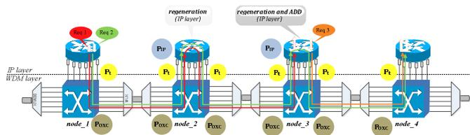
Fig. 1. Architecture of IP over flexible optical network
