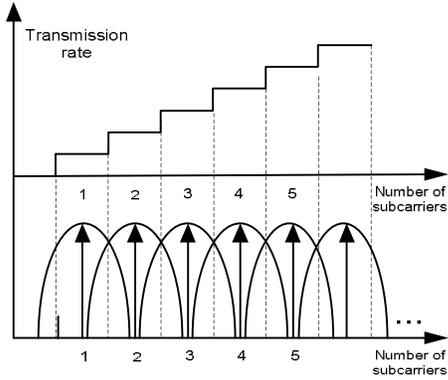
Figure 1. Variable bandwidth transmission by elastically controlling the number of OFDM subcarriers.
