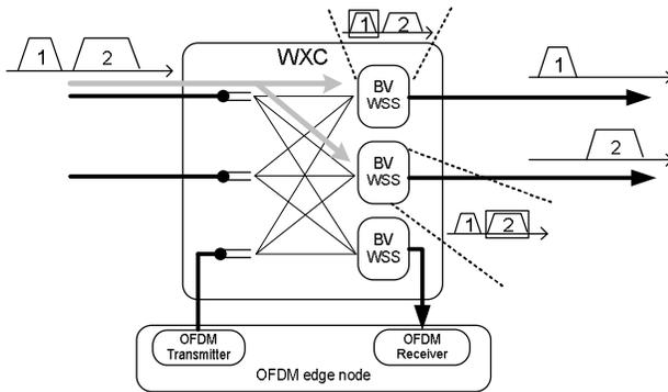
Figure 2. Spectrum flexible WXC
