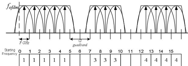
Figure 3. Spectrum allocation as a table of subcarrier slots assigned to connections. Spectrum guardaband of  $G$  subcarriers is used to separate the path flows so as to route and receive them with acceptable signal performance.
