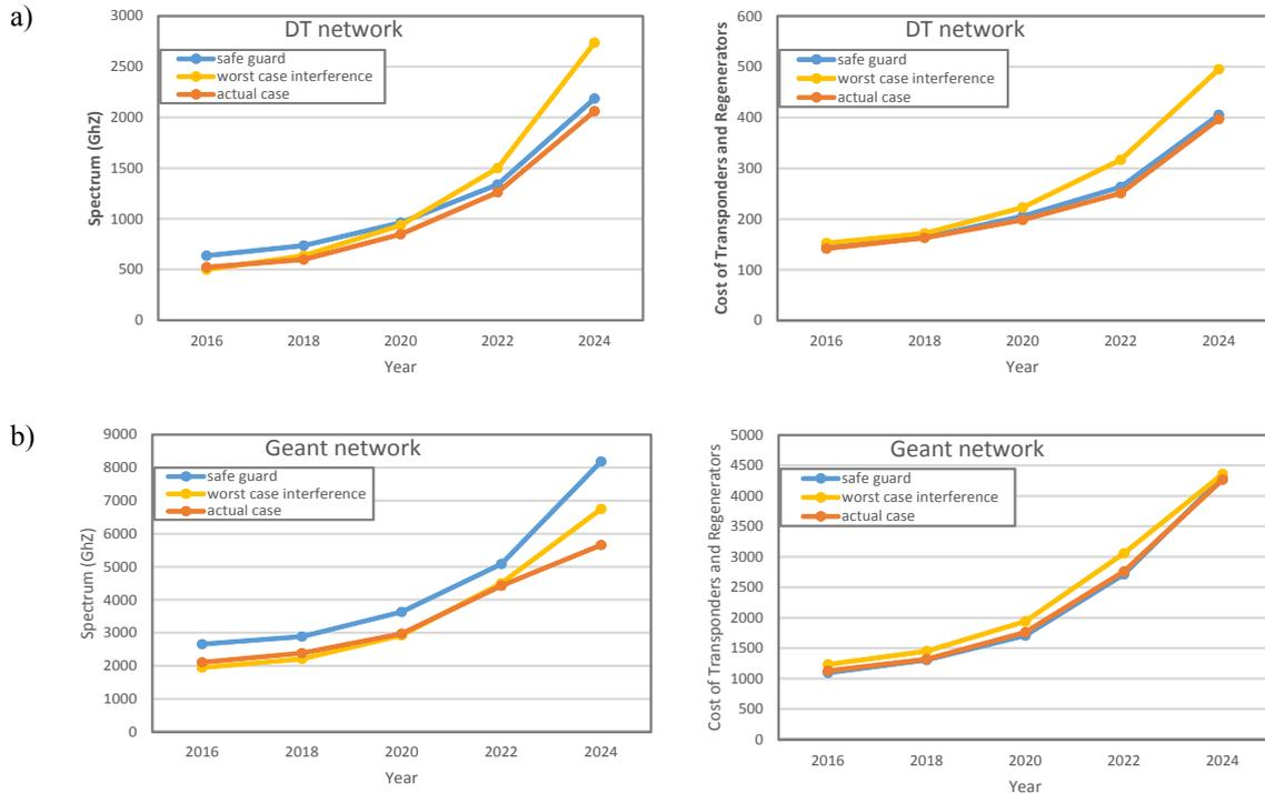
Figure 1. Spectrum utilization and cost for transponders and regenerators for: (a) DT network and (b) Geant network for the different transmission scenarios.
