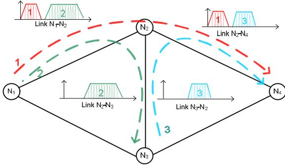
Fig. 1: Spectrum flexible OFDM-base optical network.
