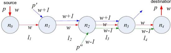
Fig. 4. Adjacent channel interference on lightpath  $(p, w)$  by other lightpaths.
