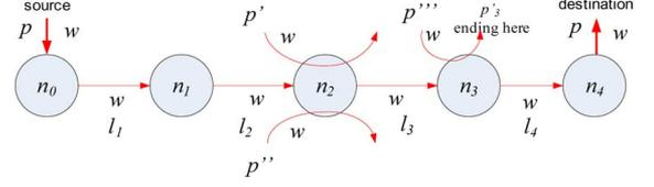
Fig. 5. Intrachannel XT interference on lightpath  $(p, w)$  by other lightpaths.
