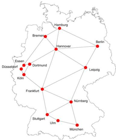
Fig. 6. Generic DT network topology (DTnet) with 14 nodes, 23 undirected links (in our simulations we assumed 46 directed links).
