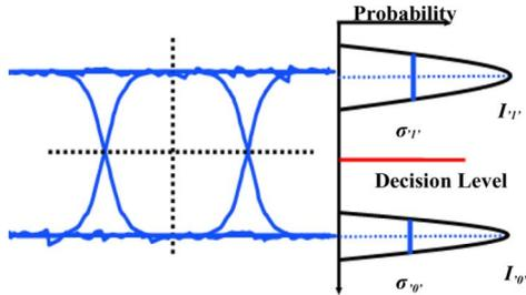
Fig. 3. Eye diagram and  $Q$ -factor.
