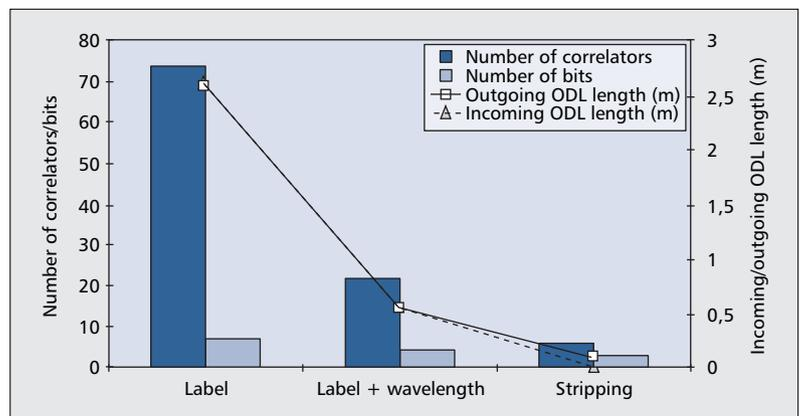
■ Figure 4. Number of components needed per wavelength for each label switching strategy.
