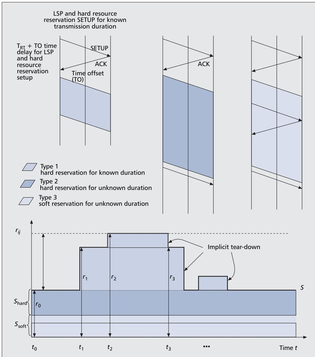
■ **Figure 6.** a) Resource reservation mechanism in combination with the LSP setup process; b) utilization profile  $r_{ij}(t)$  of wavelength  $i$  of link  $j$  at each time instance.
