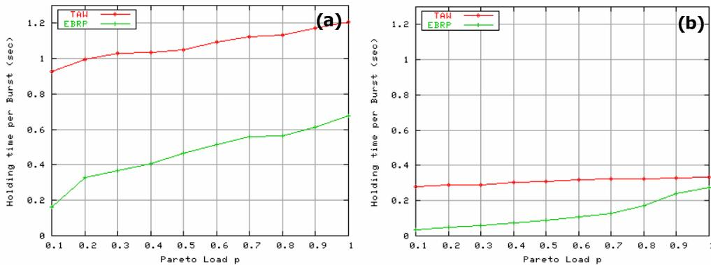
Figure 5: Average holding time at the network ingress point for the EBRP and TAW protocols for the case of (a) single and (b) multiple FIFO ER architecture. Bursts maximum allowable delays are set to infinity.
