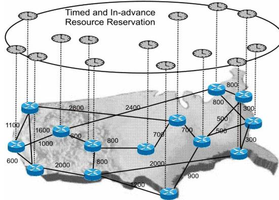
Figure 3: 14-node NSFnet backbone network topology (the shown distances are in km).
