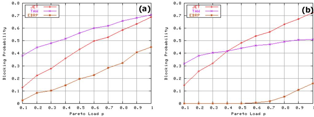
Figure 4: Blocking probability of the EBRP, TAW and JET protocol for the case of (a) single FIFO and (b) multiple FIFO ER architecture.
