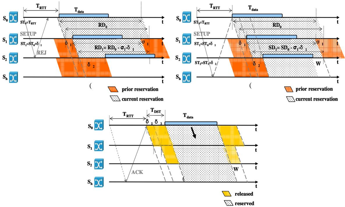
Figure 2: Timing considerations in the EBRP signaling protocol. (a) Blocked call setup phase at an intermediate node, (b) successful end-to-end call setup and (c) acknowledgement phase with abundant resources release.
