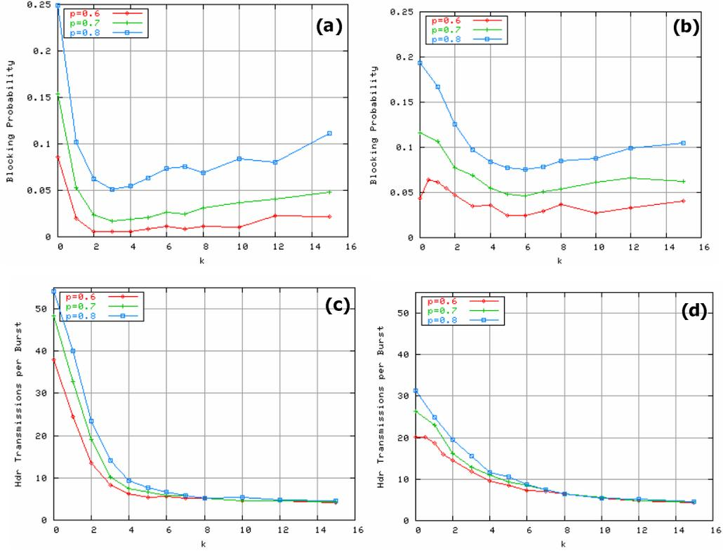
Figure 6: (a) and (b) Blocking probability for various reservation time durations values for average burst size equal to  $28.8 \cdot p$  Mbytes and  $14.4 \cdot p$  Mbytes respectively. (c) and (d) Corresponding number of SETUP retransmissions. X-axis corresponds to constant  $k$  and reservation time duration is calculated on a per burst
