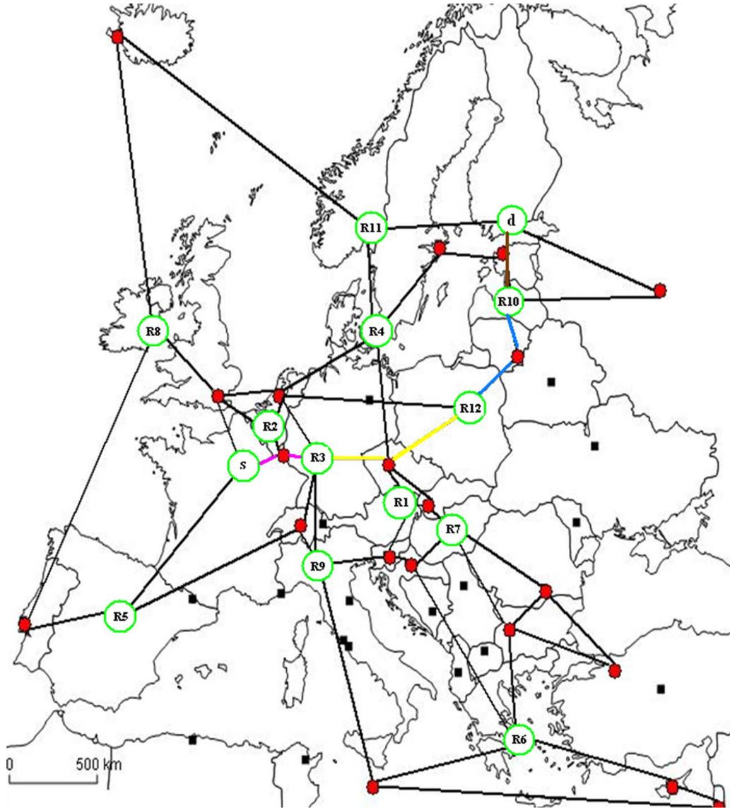
Fig. 1. Non-transparent connection request between source-destination pair  $(s, d)$  can be broken into four transparent sub-connection requests:  $s$ -R3, R3-R12, R12-R10 and R10-d. Each of the three sub-connection requests can be served using a different wavelength.
