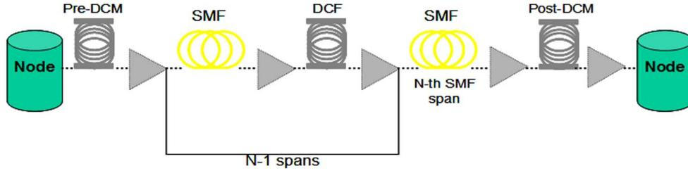
Fig. 5. Link model assumed in the experiments.
