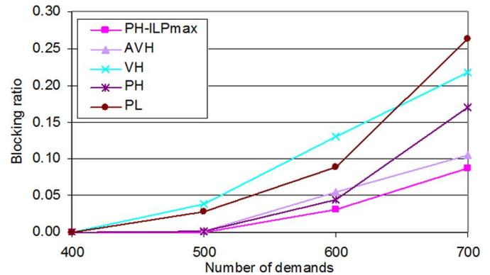
Fig. 8. Blocking ratio versus number of demands, assuming 80 available wavelengths and bounded regeneration sites and regenerators.
