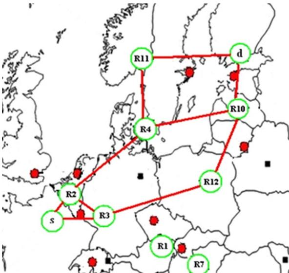
Fig. 3. Assuming regeneration sites at nodes R2, R3, R4, R10, R11 and R12, we present the related virtual topology  $\tilde{G}(s, d)$ . The source node  $s$  and the destination node  $d$  are transparently connected to regeneration sites R2 and R3, and R10 and R11, respectively.
