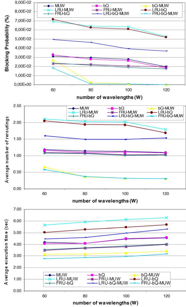
Fig. 5. (a) Blocking probability. (b) Average number of reroutings per connection. (c) Average execution time per accepted connection. All the results are presented as a function of the number of available wavelengths, for fixed network load (equal to 700 Erlangs).
