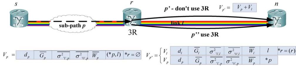
Fig. 2. Path cost vector bifurcation at a node  $r$  where a regenerator is available. A path  $p$  ending at node  $r$ , when extended so as to include link  $l = (r, n)$ , gives rise to two paths  $p'$  and  $p''$ . One of them makes use of the regenerator, while the other does not. The impairment parameters of the two paths will differ, since the path that uses the regenerator restores its signal quality, removing all impairments up to that point.
