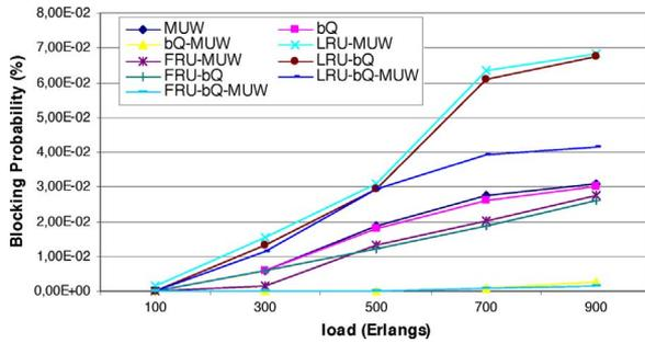
Fig. 6. Blocking probability as a function of network load. Number of wavelengths is equal to 100.
