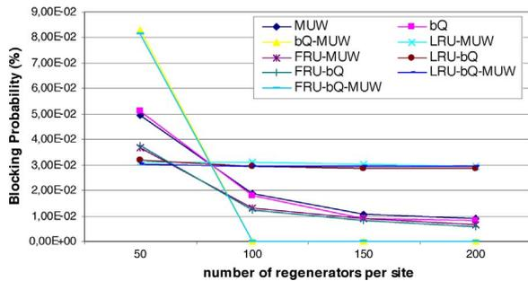
Fig. 7. Blocking probability as a function of the number of regenerators available at each site. Number of wavelengths is equal to 100 and load is equal to 500 Erlangs.
