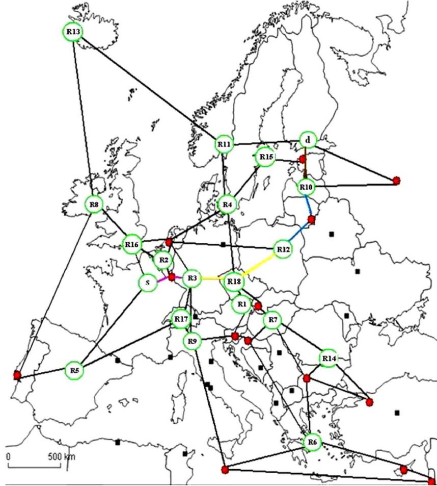
Fig. 1. Geant-2 network topology with 18 regeneration sites. The established path between the source-destination pair ( $s, d$ ) is broken into four transparent sub-paths:  $s - r_3, r_3 - r_{18}, R_{18} - r_{12}, r_{12} - r_{10}$  and  $r_{10} - d$ . Each of these five sub-paths can use a different wavelength.
